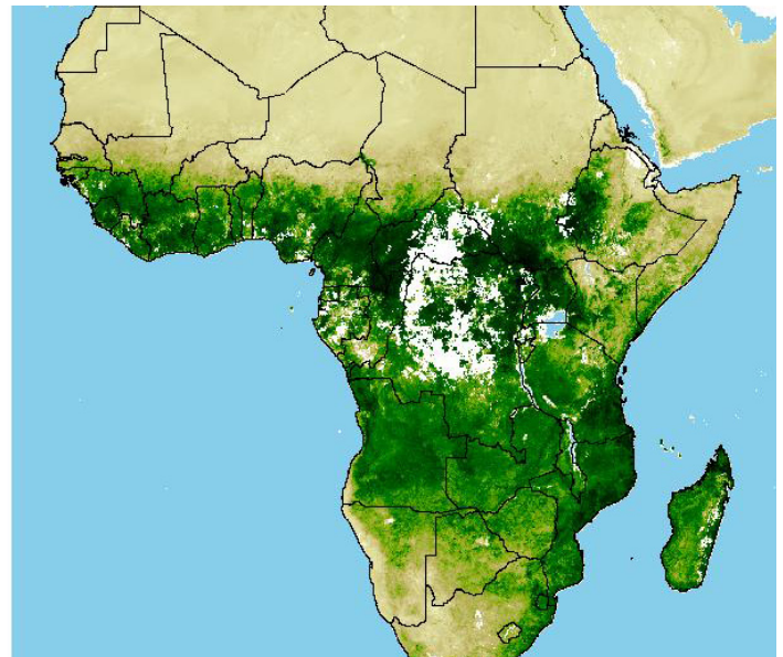
Vegetation index over Africa in May 2008 as measured by the Moderate Resolution Imaging Spectroradiometer (MODIS) instruments aboard the NASA Terra and Aqua satellites. Due to their simplicity, ease of application, and widespread familiarity, vegetation indices have a wide range of usage, including agricultural monitoring and forecasting and land-use planning. In this example, close monitoring of vegetation in regions affected by increased rainfall is used to identify areas at increased risk for outbreaks of malaria.
