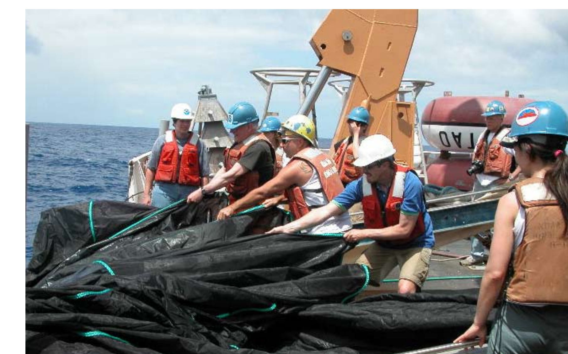
Hauling in the Data. Scientists haul in the 10 meter MOCNESS nets after a deep tow during an April 2006 cruise aboard the Ron Brown. Data sets from a MOCNESS sampling system may include zooplankton species composition, abundance, temperature, salinity, depth, and possibly oxygen, fluorescence, transmissometry and downwelling light.
