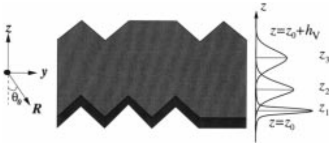
Fig. 1. Schematic representation of the random volume over ground scattering model.
