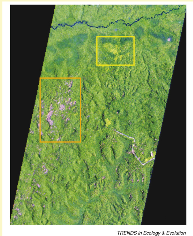
Figure 1. Blowdown gap distribution in the Central Amazon. This 2005 Hyperion image (available from the NASA LBA-ECO Project Office) shows blowdown gaps distributed across a landscape north of Manaus, Brazil, at the end of the ZF-2 road (entering from below-middle right) with shortwave-IR (1709 nm) as red, near-IR (1053 nm) as green, and visible red (650 nm) as blue. Owing to spectral reflectance differences in exposed wood and surface litter in blowdown gaps, these patches show up as red–blue (orange box). An old blowdown, with regrowing vegetation showing strong reflectance in the near-IR, shows up as bright green (yellow box), but with the clear blowdown pattern characterized by Nelson et al. [89]. Quantitative disturbance maps can be developed from this image by applying SMA methods similar to those used to detect logging [10,11]. In contrast to existing forest inventory methods, stratified random sampling across this entire disturbance gradient will enable researchers to address important questions regarding controls over species distribution and abundance, and landscape carbon balance. [ED: please move figure to Box 4].
